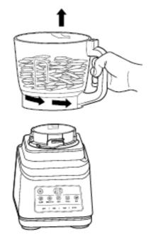
11. To remove the bowl from the motor base, turn the bowl anticlockwise and then lift it.
