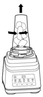
6. To remove the cup from the motor base, turn the cup anti-clockwise and then lift up.
