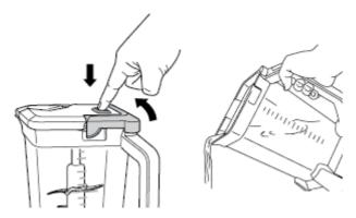
8. For thicker mixtures that cannot be emptied through the pour spout, remove the lid and Stacked Blade Assembly before pouring. To remove the lid, press the RELEASE button and lift the handle. To remove the blade assembly, carefully grasp it by the top of the shaft and pull straight up. The Jug can then be emptied.
