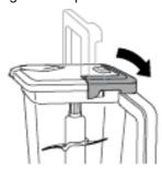
5. Place the lid on the Jug, aligning the triangle symbol on the lid with the triangle symbol on the handle. Press
