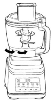
7. To remove the bowl from the motor base, turn the bowl anti-clockwise and then lift up.
