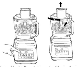
8. When finished, stop the unit by touching the Power button and wait for the disc to stop spinning. Press the button on the feed chute lid near the handle to unlock, then turn the lid anticlockwise. Lift the lid from the bowl.
