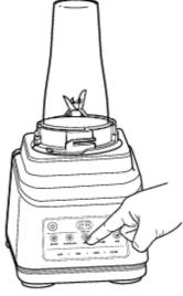
5. If using an Auto-IQ® program, first select the program that best suits your recipe. The preset feature will automatically stop at the end of the program. To stop the unit at any time, press the currently active program
