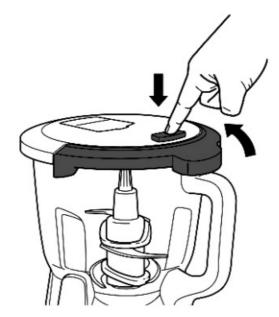
Remove the lid by pressing the RELEASE button on the front tab and then lifting up on the handle. Always remove the Chopping Blade Assembly before emptying the ingredients from the bowl. To remove the Chopping Blade Assembly, carefully grasp it by the top of the shaft and lift it out of the bowl.
