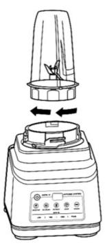
4. Turn the cup upside down and install on the motor base. Align the tabs on the cup with the slots on the base, then rotate cup clockwise until it clicks into place. Once the cup is locked in place, press the Power button to turn unit on. The available program buttons will illuminate and the unit will be ready for use.
