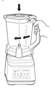
2. Lower the Total Crushing Pitcher onto the motor base. The handle should be aligned slightly to the right and the pitcher should be oriented so the LOCK symbols are visible on the motor base, Rotate the pitcher clockwise until it clicks into place,
