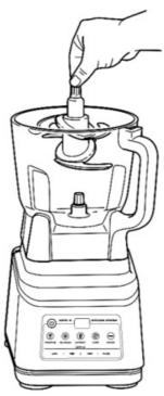
3. Exercising care, grasp the Chopping Blade Assembly by the top of the shaft and place it onto the drive gear inside the bowl. Note that the Chopping Blade Assembly will fit loosely onto the drive gear.
