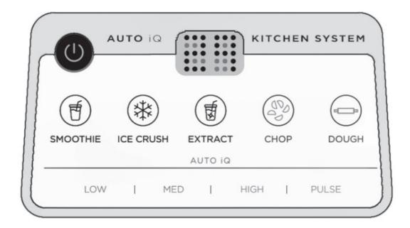
**NOTE**: The unit can detect which container is installed on the motor base. Only the functions available for a particular container will illuminate on the control panel.
