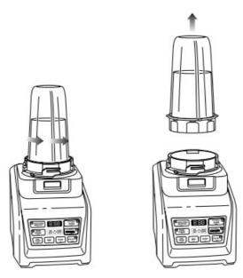
7. Once you have reached your desired consistency, stop the appliance by pressing the power button and wait for the Pro Extractor Blades Assembly to stop turning. Turn the Nutri Ninja Cup anticlockwise and pull straight up to remove it.
