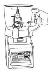
5. Rotate the bowl clockwise until it locks in place, you will hear a click when the lock is engaged.
