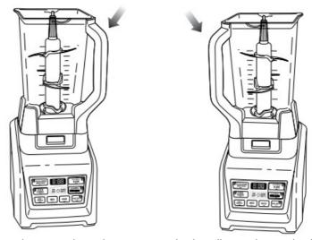
6. The pitcher can be placed on the motor base in two ways; the handle can be on the front right corner or the front left corner.
