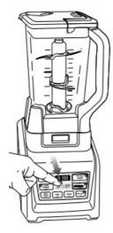
11. Press the power button to turn on the unit. Select the speed or Auto-iQ program that best suits your needs. The Auto-IQ program will stop the appliance automatically at the end of the program.
