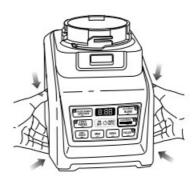
18. To release the motor base from the counter or tabletop, place your hands underneath both sides of the motor base and gently pull the unit up and towards you.
