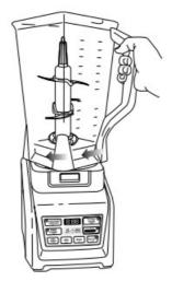
5. Rotate the pitcher clockwise until it locks in place, you will hear a click when the lock is engaged.
