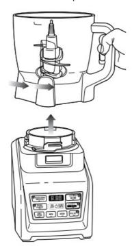
7. Turn the bowl anticlockwise and lift it to remove it from the motor base.
