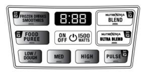
NOTE: Nutri Ninja | Ninja Blender System with Auto-IQ Technology can sense which jar is on the motor base. The available function lights will illuminate depending on which jar is placed on the motor base.
