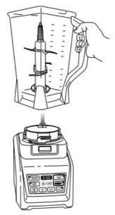
4. Align and lower the pitcher onto the motor base. The handle should be aligned slightly to the right of the LOCK symbol on the motor base.
