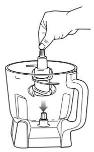
2. Holding the desired blade by the top of the shaft, place it onto the drive gear inside the bowl. Ensure that the attachment is seated properly and is standing upright.
