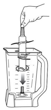
2. Holding the Stacked Blade Assembly by the top of the shaft, place it onto the drive gear inside the pitcher. Ensure that the Stacked Blade Assembly is seated properly and is standing upright.
