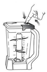
16. For thicker consistencies, first, remove the lid by pressing the release button and pulling the lid handle up to a 90-degree angle to lift lid off the pitcher.
