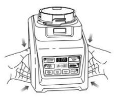
8. To release the motor base from the counter or tabletop, place your hands underneath both sides of the motor base and gently pull the unit up and towards you.
