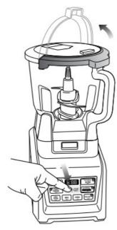
5. To remove the lid, press the release button on the lid and pull the lid handle up to a 90-degree angle.
