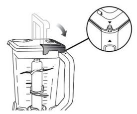
8. Holding the lid by the handle in the upright position, place it on top of the pitcher aligning the triangle located on the lid with the triangle ▼ located on the pitcher's handle. Press the handle down until you hear a click. The triangles ▲ on the lid and the blender handle MUST be aligned in order for the blender to turn on.
