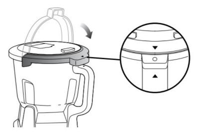
8. Holding the lid by the handle in the upright position, place it on top of the Processor Bowl aligning the triangle located on the lid with the triangle located on the Processor Bowl handle.
