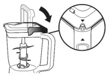
5. Place the lid on the pitcher, aligning the triangle symbol on the lid with the triangle symbol on the handle. Press down on the handle until it clicks into place. The triangle symbols MUST be aligned for the lid to lock and the unit to operate. Once the lid is locked in place, press the Power button to turn unit on. The available program buttons will illuminate, and the unit will be ready for use.
