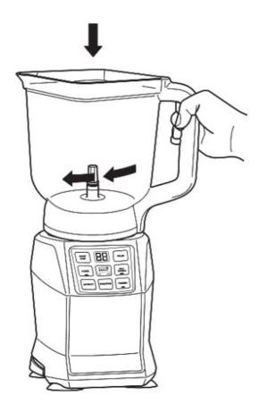
2. Lower the \*Total Crushing Pitcher onto the motor base. The handle should be aligned slightly to the right and the pitcher should be oriented so the LOCK symbois are visible on the motor base. Rotate the pitcher clockwise until it clicks into place.
