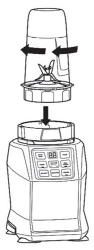
4. Turn the cup upside down and install on the motor base. Align the tabs on the cup with the slots on the base, then rotate cup clockwise until it clicks into place. Once the cup is locked in place, press the Power button to
