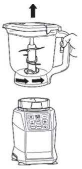
7. To remove the pitcher from the motor base, turn the pitcher counterclockwise and then lift it.
