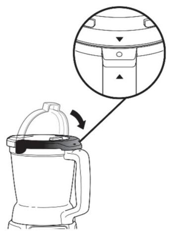
5. Place lid on the bowl, with black line on tab aligned slightly to the right of tab on front of the bowl. Turn lid clockwise to lock in place. When properly locked, the white line on lid will line up with the black line on bowl. Once the lid is locked in place, press the Power button to turn unit on. The available program buttons will illuminate and the unit will be ready for use.
