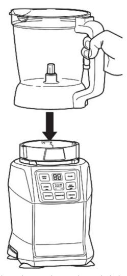
2. Lower the Precision Processor Bowl onto the motor base and rotate it clockwise until it clicks into place.
