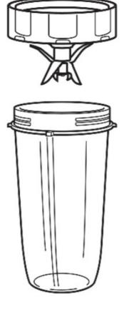
3. Install the Pro Extractor Blades® Assembly onto the top of the cup. Twist the lid clockwise until it's sealed tightly.
