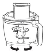
8. Release the lid by twisting anti-clockwise and lifting upwards from the motor base. Ensure the blade is removed before emptying the contents.
