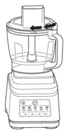
5. Place the feed chute lid on the bowl and turn clockwise until you hear a click, indicating the lid is locked in place.
