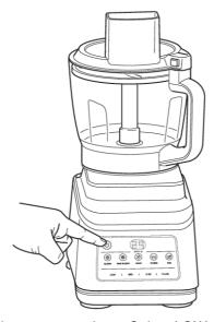
6. Plug in the unit, then press the Power button to turn it on. Select LOW. The disc will begin spinning.
