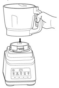
2. 2 Lower the Food Processor Bowl onto the motor base and rotate clockwise until it clicks into place.
