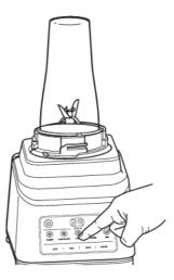
5. If using an Auto-IQ® program, first select the program that best suits your recipe. The preset feature will automatically stop at the end of the program. To stop the unit at any time, press the currently active program again. If using a manual program, select your desired speed. Once the incredients have reached your desired consistency, press the active button again, and wait for the unit to come to a complete stop.
