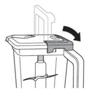
5. Place the lid on the Jug, aligning the triangle symbol on the lid with the triangle symbol on the handle. Press down on the handle until it clicks into place. The triangle symbols MUST be aligned for the lid to lock and the unit to operate. Once the lid is locked in place, press the Power button to turn unit on. The available program buttons will illuminate and the unit will be ready for use.
