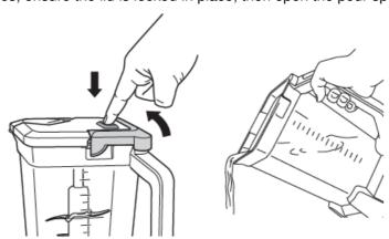
For thicker mixtures that cannot be emptied through the pour spout, remove the lid and Stacked Blade Assembly before pouring. To remove the lid, press the RELEASE button and lift the handle. To remove the blade assembly, carefully grasp it by the top of the shaft and pull straight up. The Jug can then be emptied.
