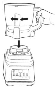
2. 2 Lower the Food Processor Bowl onto the motor base and rotate clockwise until it clicks into place.
