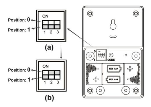
There are 3 sliding switch handles, and mentioned numbers 1, 2 and 3 on the switch. Each switch handle can move to 2 positions UP and DOWN. UP represents 0 position and DOWN represents 1 position. The factory default mode is Automatic mode (111), and the three switch handles is at 1 position (see fig (a)). For example, when you want to choose Delay-off 8H mode (100), just move the switch handle 2&3 to 0 position (see fig (b)), then setting finished. Other mode settings, and so on.
