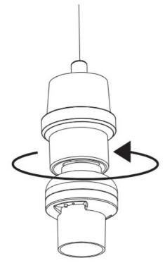
2. Remove the isolation tab in the battery compartment of the transmitter.
