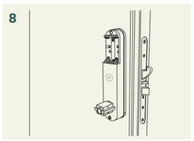
9. Fit the inside of the lock by fastening both the screws in the battery holder and the one at the bottom. Install all batteries and the battery cover.
