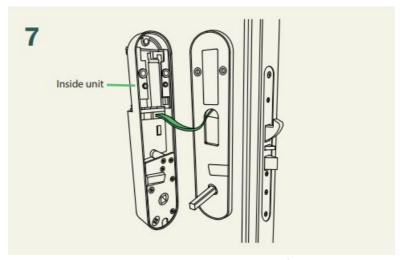
8. Insert the excess cord into the door to prevent it from getting caught. Slide the inside unit into place.
