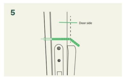
6. Adjust the cuttable screws so that they correspond to the thickness of the door and add an extra threaded portion. Use powerful pliers to cut to the desired length. The length should be equal on all screws. Cut further if necessary.
