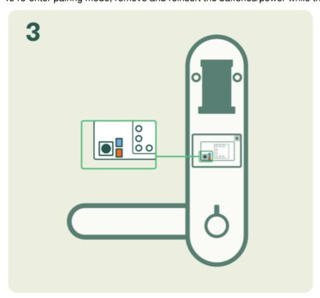
How to reset: hold down the reset button on the module until the orange indicator blinks rapidly (about 15 seconds). Release the button immediately.
