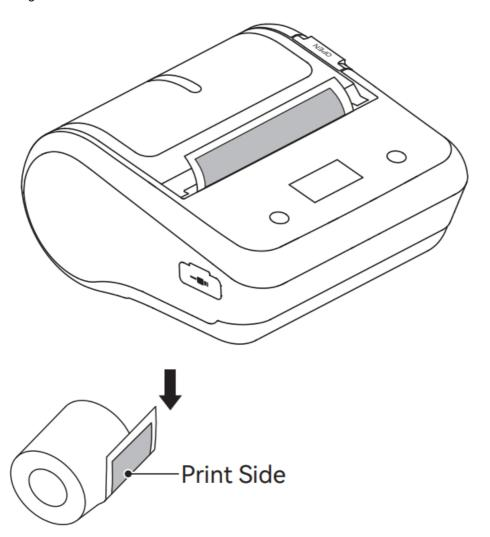
**Note**: The print paper should be installed into the compartment with the print side facing down.
