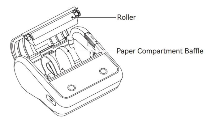
4. Fit the print paper into the compartment with the print side facing down, and the first label paper sticking out of the tear-off opening, and then close the compartment.
