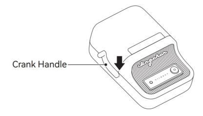
1. Press down the crank handle on the left side of the device to open the paper compartment.
