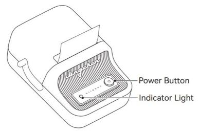
3. Close the paper compartment cover and long-press the power button to switch on the device.
