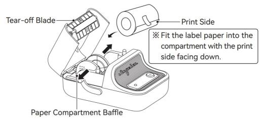
2. Push the paper compartment baffle to both sides and fit the label paper roll down into the compartment.
