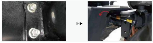
4. If you are installing a winch, remove the frame cover. This requires removing the center pin from the two clips, then pulling the clips out or some prefer to leave it on if not running a winch, with applicable bumpers.
