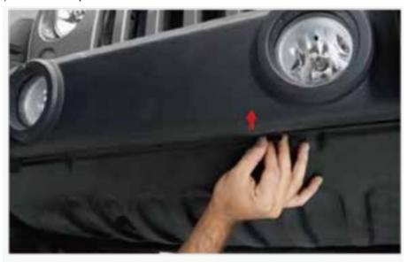
2. Remove the factory fog light connections by pushing the tab in on the brown connector and gently pulling out.
