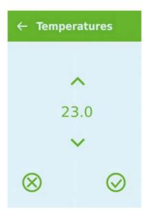
If you select the option of current room temperature, the desired room temperature will be displayed. The desired room temperature can be adjusted by pressing the up-or-down arrows followed by the cancel icon (bottom left) or the accept icon (bottom right).
