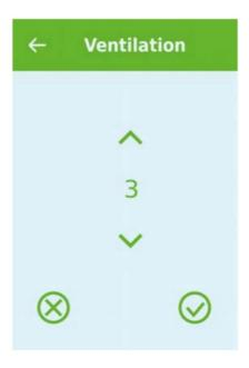
If you select the option of current fan speed level, the desired fan speed level will be displayed. The desired fan speed level can be adjusted by pressing the up-or-down arrows followed by the cancel icon (bottom left) or the accept icon (bottom right).
