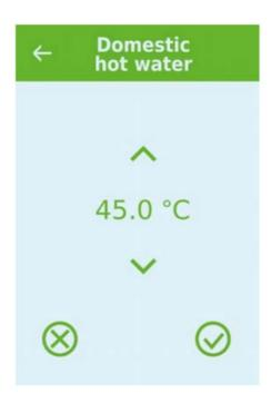
By pressing the current hot water temperature the desired hot water temperature is displayed. The desired hot water temperature can be adjusted by pressing the up-or-down arrows followed by the cancel icon (bottom left) or the accept icon (bottom right).
