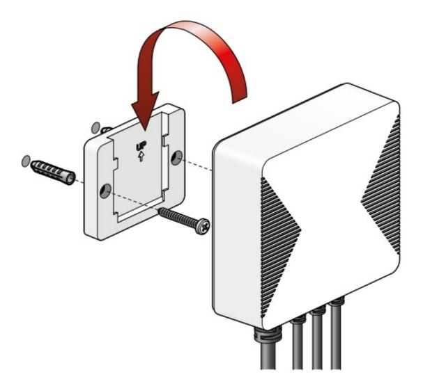
All cable inserts in the electrical cabinet need to be sealed off. The method to close off the cable entries is defined by national installation
