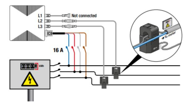
This product must be secured with a miniature circuit breaker (MCB) of max. 16 A in the electrical cabinet. The MCB rating is limited by national installation rules.
