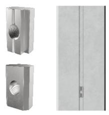
Back of Aluminium gauge board showing M6 Tee nut which slides and can be fixed at any point on the gauge board making it practical and simple to install to tank.
