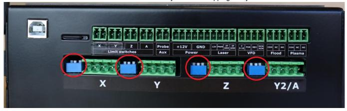
A small pick or screwdriver can be used to set the micro-stepping from the front of the unit or the controller cover can be removed to make setting the values easier, see below for removing cover.
