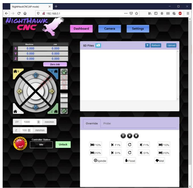
To start configuring your controller Click on the "Settings" button at the top right. This will expose the network configuration options and general CNC settings. It is possible from the Web portal to configure any settings you would like to change imcluding your connection type.
