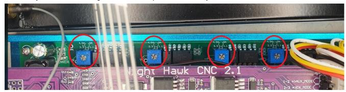
Each dial has a guide above it to indicate roughly what the current setting is. The quick method for setting your current is by visually adjusting the dial using a small Phillips head screw driver. See diagram below of where the indicator is, there are 2 notches either side of it. See also below the approximate value of each chevron on the dial:
