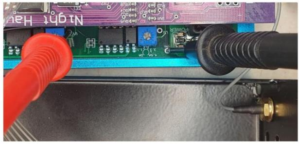
Once your multimer probes are in position and a voltage is showing, use a small screw driver to carefully turn the blue dial being set, rotate clockwise to increase current and counter-clockwise to decrease the current. While turning, check the voltage change on your multimeter for the expected value.
