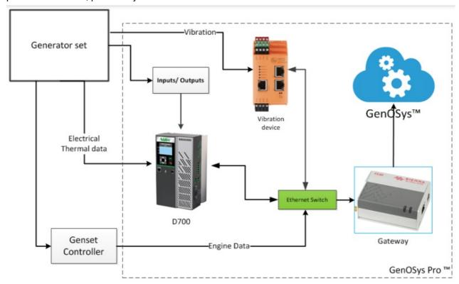
It's an easy-to-install, box-integrated solution. The architecture is shown below and is suitable for small and medium power installations. This solution interfaces with digital voltage regulators type D550 to collect electrical data.
