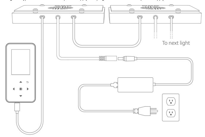
**NOTE** For HyperReef Gen 1, use 3.5mm TRRS Audio Cables to connect lights (HyperReef 50/100/ 150) to the controller and to daisy-chain the lights together. (Cables not included)
