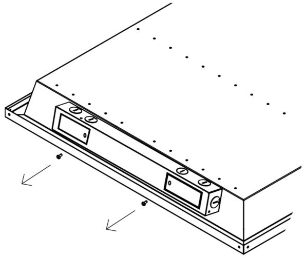
6. Connect wiring as shown. Grey and purple wiring are for 0-10V dimming systems. Cap off if not used.
