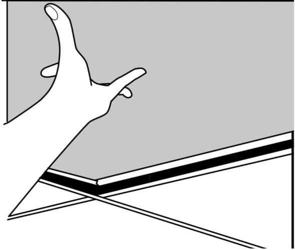
5. Remove the access plate from the junction box (do not discard it) by removing the screws. Another end is for low voltage connection.
