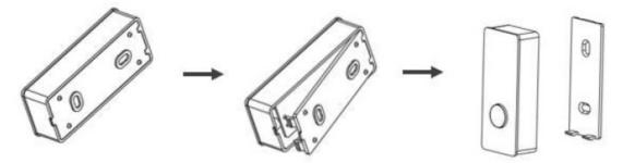
3. Screw the bottom cover to the wall
