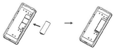
5. Hook the Button with battery onto the wall mounted bottom cover.
