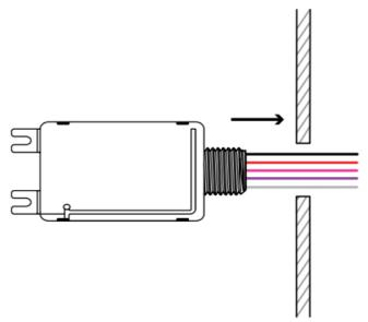
4. Place lock-nut over the wires and screw onto threading to tighten controller.
