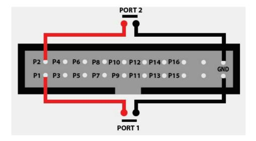
To activate a port, a brief contact of at least 1/25 second must be established between the ports (1...16) and the ground (GND) using the external HE20 connector. A suitable IDC cable can be found by searching for 'IDC 20 Pins Connector Flat Ribbon Cable Female Connector 2.54mm Pitch'. If making your own cable you will need '20 Way Flat Ribbon Cable, Pitch 1.27mm'. To connect cable to a screw terminal breakout board, search for 'IDC20 2×10 Pins Male Header Breakout Board'.
