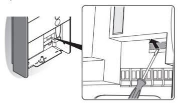
5. Insert the BiDi-ZWave into the BUS T4 port of the connector unit
