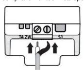
4. If present, remove the plastic pre-cut element from BUS T4 connector and check that there are no burrs
