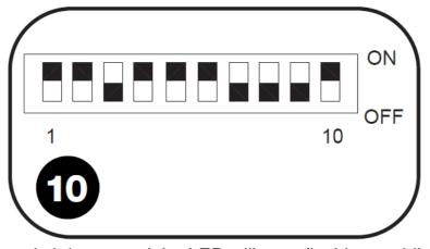
4. After the 10th dip switch is entered the LED will start flashing rapidly for 5 seconds. If no button is pressed while the LED flashes, the code will be memorised, otherwise the operation will be cancelled.
