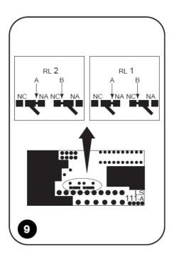
In the FLOXM and FLOXM220 versions, proceed as described in points 2 and 3 on the solder side of the relay units (fig.8).
