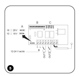
Make sure the power input mode is correct before powering the receiver. In all the versions, the receiver outputs are normally open (N.O.) pure contacts provided by the relays on the board. In the FLOXM and FLOXM220 versions, the outputs are provided through the plug-in relay units (ref. M fig.6); there are three kinds of relay unit:
