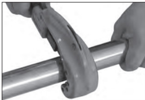
Figure 1 — Cut tube to desired length
