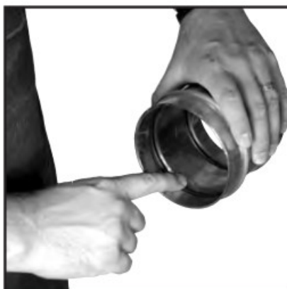
Figure 5: Check for EPDM seal
