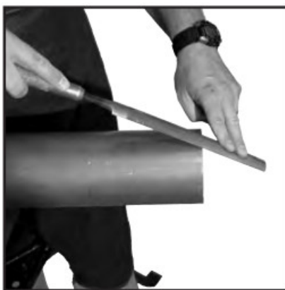
Figure 4: Deburr outside diameter using a half-round file
