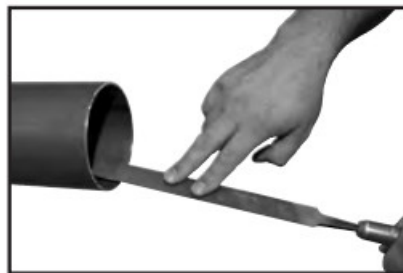
Figure 2: Deburr inside diameter using a half-round file
