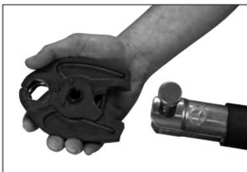
Figure 5 — Inserting the NIBCO Press System jaw
