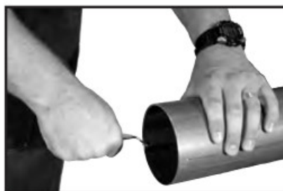
Figure 3: Deburr inside diameter deburring tool
