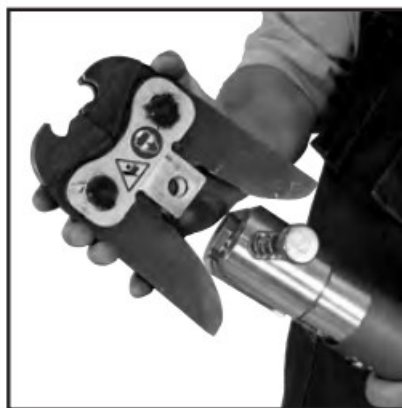
Figure 7: Placement of adapter jaw into the tool
