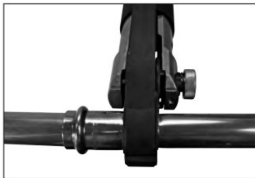
Figure 8 — Jaw set should be square to tubing
