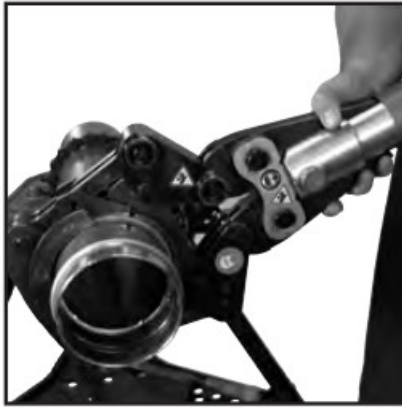
Figure 8: Placement of adapter jaw into pressing chain
