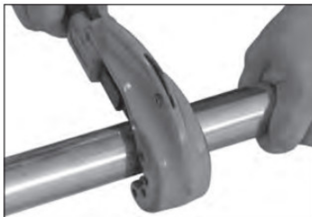
Figure 1 — Cut tube to desired length
