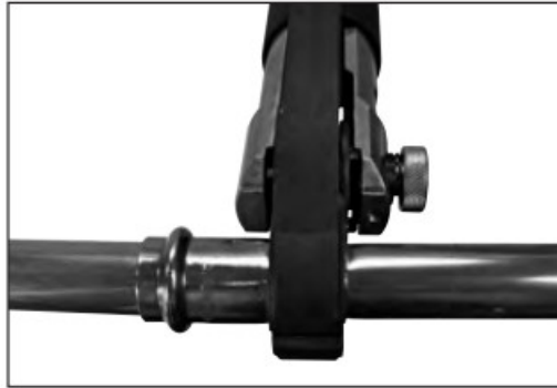
Figure 8 — Jaw set should be square to tubing
