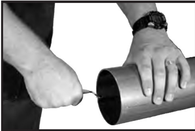
Figure 3: Deburr inside diameter deburring tool
