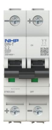
Suitable for panelboards with DC compatible busbar chassis (2P). Red/green contact position indicator that is independent of the toggle position. Inbuilt permanent magnet to ensure quick arc extinguishing. Quick install into Concept distribution panelboards.
