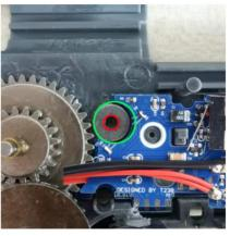
The green circle indicates the detection position of DTU gear sensors, and the red circle indicates the rotation axis position of sector gear. When DTU matches the position of gearbox, the centers of the two circles will coincide.
