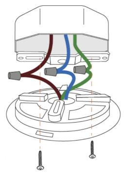
4. Fit the lamp and the ceiling plate together and slightly rotate the lamp clockwise. After this, your ceiling lamp will be secure and ready for use.
