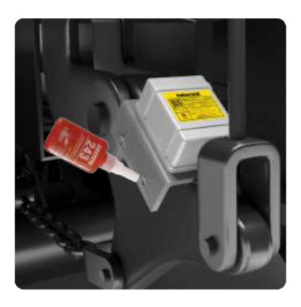
Use the 5/32" hex key to tighten all three set screws. Make sure the Vector Sensor remains centered in the bellcrank. Note: Ensure the set screws are pressing firmly against the bellcrank and not caught on the lip.
