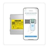
Hold smartphone NFC to the Vector sensor to verify connection and initiate the pairing process.
