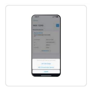
Hold smartphone NFC to the Loadtracker sensor to verify connection and initiate the pairing process.
