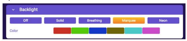
In Marquee Mode, you can set the led color of each tube and the color will change in a loop one by one.
