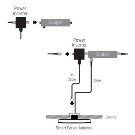
**STEP 3:** Drill a 2-inch (50 mm) diameter hole in the dropped ceiling at the desired Smart Server Antenna location. **NOTE:** If installing on a hard ceiling, go to Step 3 in the "HARD CEILING INSTALL" section.
