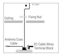
**STEP 5:** Thread the DC Power cable through the Fixing Nut above the ceiling and down through the hole. Continue by guiding it through the center of the Dropped Ceiling Mounting Plate, ensuring that the DC cable wires extend with sufficient length for easy connection to the DC wire terminal block on the antenna.
