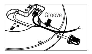
**STEP 7:** Align the plastic clips on the Hard Ceiling Mounting Plate with the three holes on the antenna and snap the antenna onto the plate in the direction of the cable groove.
