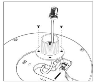
• STEP 5: Thread the DC Power cable through the Fixing Nut above the ceiling and down through the hole. Continue by guiding it through the center of the Dropped Ceiling Mounting Plate, ensuring that the DC cable wires extend with sufficient length for easy connection to the DC wire terminal block on the antenna.
