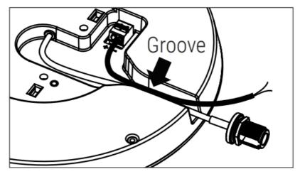
• STEP 5: Align the plastic clips on the Hard Ceiling Mounting Plate with the three holes on the antenna and snap the antenna onto the plate in the direction of the cable groove.
