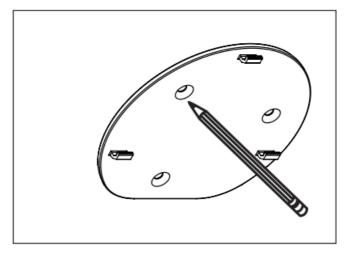
• STEP 2: Drill the three holes for the supplied Drywall Anchors.
