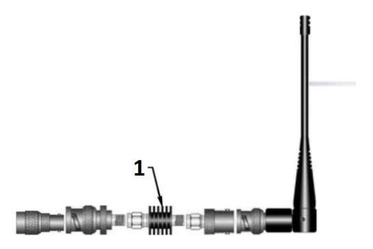
**Note:** It is important to use attenuation between all demo units in the test network to reduce the amount of signal strength in the test environment.
