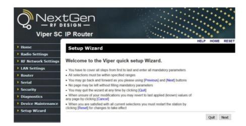
The Setup Wizard consists of five (5) steps. Each step is presented as a single page with a few simple options to fill in or select from. Each of the five pages for each step of the Setup Wizard contain the basic configuration settings that are most required to select or change to set up the Viper SC+ IP router for specific functionality.
