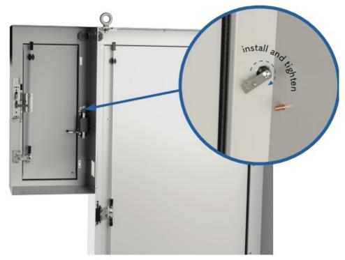
4. Install the two mounting brackets (item 8). One to the interior side wall of the external disconnect and one of the main enclosure using ½-20 flange nuts (item 1) (Two each).
