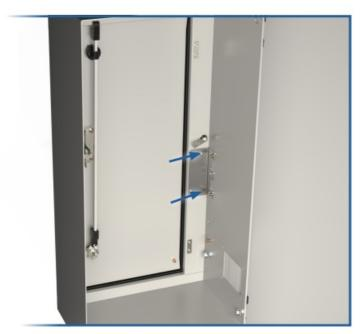
5. Install primary interlock (item 6) into NEXD enclosure and secondary door interlock (item 7) in main enclosure with 10-32 flange nut (item 2) to mounting bracket. Hold interlock at highest point on the stude and tighten place
