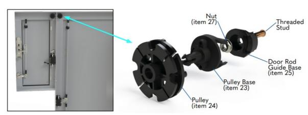
• Drill a 0.25" mounting hole into the top flange of the main enclosure (see image below for location) for installation of door rod guide base (item 25). Install using 1/4-20 button head screw (item 4) and sealing washer (item 5).
