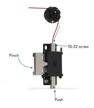
10. Adjust to increase tension by loosening the 10-32 nuts on interlock and push down as needed. Then retighten nuts. This will allow for the locking arm to move in farther.
