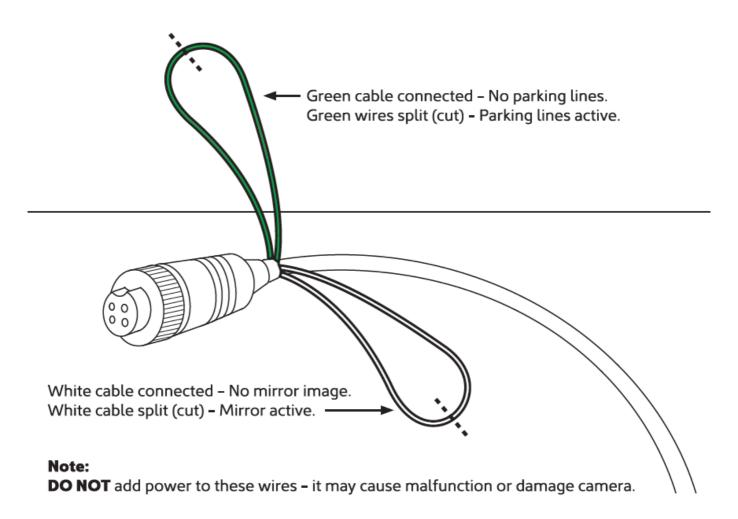
**Note:** DO NOT add power to these wires – it may cause malfunction or damage camera.
