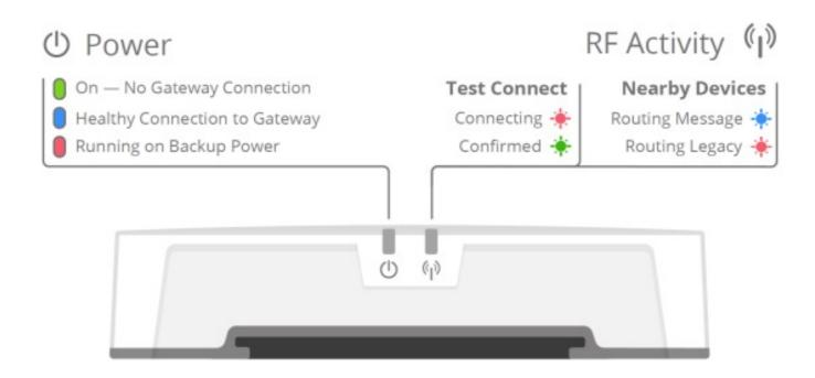
**Note:** After the Test Connect button is pressed, two slow blinks of the RF Activity LED show whether the Gateway can be reached. Fast blinks will occur at any time as signals are received from nearby NextCentury devices.
