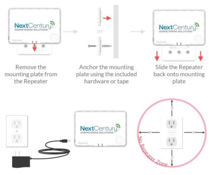
Power the Repeater using the included power supply
