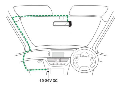
The Dash Cam will automatically power on and start recording once power is available. In some vehicles this will be when connections are made, for others the Dash Cam will power on once the ignition has been turned on.
