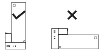
**5** Orient the battery packs so that the diagonal stripes are facing the locking tabs with the metal contacts facing towards the inside of the Side Dock Charge station. Carefully slide the battery packs into the charge station until they lock in place.
