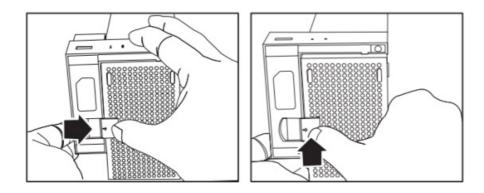
**4** Gently press the Side Dock Charging Station against the Xbox Series S to assure there is solid contact between the mounting pad and the console.
