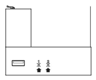
**6** When the battery pack is fully charged, slide the locking Unlock switch up to unlock. The battery automatically pops out.
