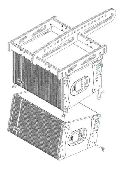
• Step 5 – Insert the next LA122 in the array starting with the front side and insert the front locking pins. Check if the locking pins are secured.
