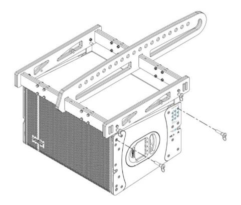
• Step 3 – Insert a locking pin on both front swivel arms first, then lift the frame at the back until the swivel arm is aligned with the 0° hole. Insert now lock pins at these holes on both sides of the element and verify they're secure.
