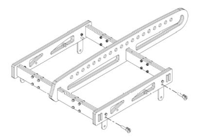
Step 1 – Pull the frame's swivel arms out of the parking position and insert a safety
