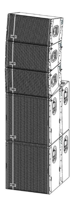
The LA122W2 is a little different from the LA122v2. The principle is the same, but instead of eight possible splay angles, it has only two splay positions, which differ according to the element that is mounted above it. When it is assembled below a LA1222, for example as a nearfield speaker, the position will be 11.5°. When coupled to another LA122Wz, the position will be 15°. We can see this information on the panels of the element as shown below.
