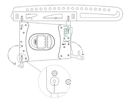
**Step 4** – Pull the LA122vz swivel arms out. On the front swivel arms, insert the locking pin. This will assure that the centre of rotation of the next element is fixed. Check if the locking pin is secured.
