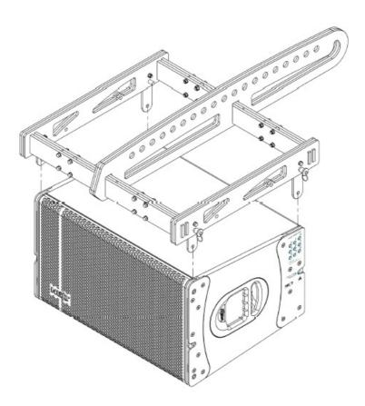
• Step 2 – With the swivel arms locked in place, align and insert them in the LA122v2 as shown above.
