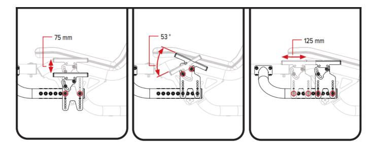
Loosen or remove the Bolts indicated above and change the Shifter & Handbrake Plate Assembly to your desired Height, Angle and Position. Retighten or reinstall the Bolts to lock in place.
