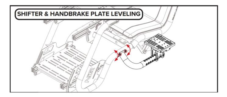
If Shifter & Handbrake Plate is tilting away from cockpit, loosen all 4 Shifter Arm mounting Bolts, pull upwards on Shifter Arm until Shifter Plate is level. Tighten Shifter Arm mounting Bolts whilst holding upwards tension.
