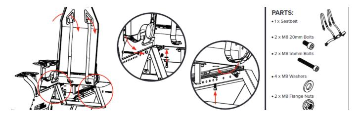
Thread the Seatbelt through the eyelets in the Seat Backrest. Align the mounting holes on each Seatbelt mounting plate with the through holes on the Seat Frames and the threaded inserts on the underside of the Seat Bottom. Bolt through and secure with 4 x M8 Bolts, Washers and 2 x M8 Flange Nuts.
