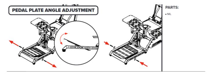
Uninstall the front Bolts, Square Washers and Flange Nuts securing the Pedal Angle Plate to the Pedal Frame and loosen the rear Bolts. Adjust to the desired angle. Bolt through and secure with the Bolts, Square Washers and Flange Nuts previously uninstalled.
