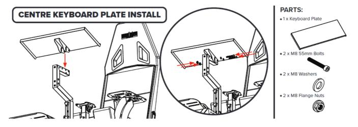
Align the mounting holes and slots on the Keyboard Plate with the through holes on the Centre Inner Pole. Bolt through and secure with  $2 \times M8$  Bolts, Washers and Flange Nuts.
