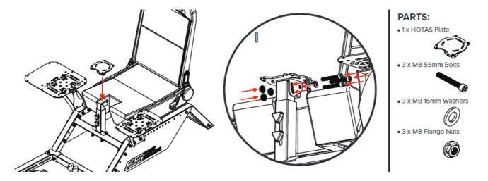
Align the mounting holes on the HOTAS Plate with the through holes on the HOTAS Inner Pole. Bolt through and secure with  $3 \times 10^{-2}$  x M8 Bolts, Washers and Flange Nuts.
