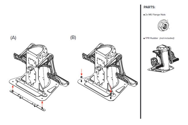
Align the mounting holes on the front of the TPR Rudder with the Threaded Studs on the TPR Adaptor. Secure with  $2 \times M6$  Flange Nuts. The TPR Rudders are ready to install onto the cockpit.
