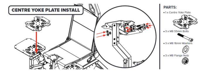
Align the mounting holes on the Centre Yoke Plate with the through holes on the Centre Inner Pole. Bolt through and secure with 3 x M8 55mm Bolts, Washers and Flange Nuts.
