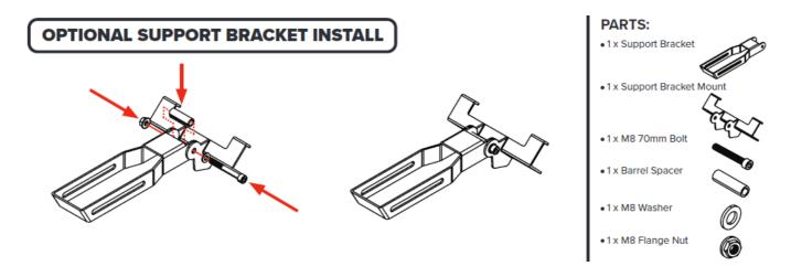
Align the pivot point on the Support Bracket with the mounting holes on the Support Bracket Mount. Bolt through and secure with  $1 \times M8$  Bolt, Washer, Barrel Spacer and Flange Nut.
