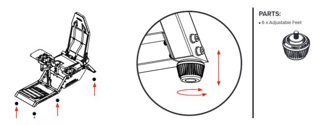
Align the Adjustable Feet with the threaded inserts on the bottom of the Pedal Frame and Seat Frames. Lock into place by twisting the Adjustable feet into the threaded inserts. To raise an Adjustable Foot, twist anti-clockwise.
