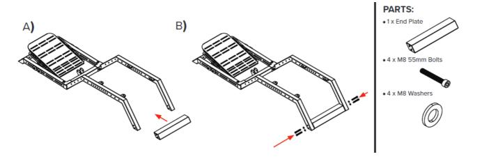
Align the threaded inserts on the End Plate with the mounting holes on the Left and Right Seat Frames. Bolt through and secure with  $4 \times M8$  Bolts and Washers.
