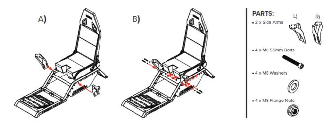
• Align the mounting slots on the Left and Right Side Arms with the through holes on the Left and Right Seat Frames and Side Panels.
