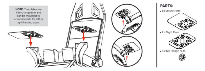
Align the Threaded Studs on the Mouse Plate and Flight Plate with the mounting holes on the Left and Right Side Arms. Secure with 8 x M8 Flange Nuts.
