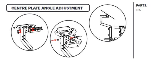
Uninstall the front Bolts, Washers and Flange Nuts securing the Centre Plate to the Inner Centre Pole. Angle to the desired position. Bolt through and secure with 1 x Bolt, Washer and Flange Nut previously uninstalled.
