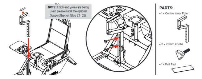
Install 1 x Felt Pad onto the top of the Centre Inner Pole. Align the threaded inserts on the Centre Inner Pole with the slots on the Centre Outer Pole. Bolt through and secure with 2 x Knobs.
