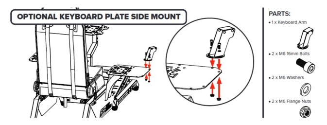
Align the mounting slots on the Keyboard Arm with the holes on the Mouse Plate. Bolt through and secure with 2 x M6 Bolts, Washers and Flange Nuts.
