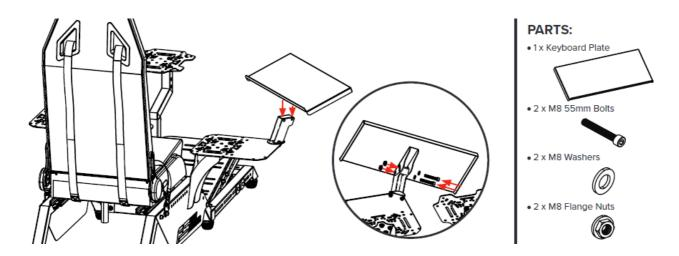
Align the mounting holes on the Keyboard Plate with the through holes on the Keyboard Arm. Bolt through and secure with 2 x M8 Bolts, Washers and Flange Nuts.
