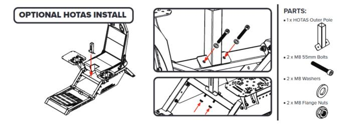
Align the mounting holes on the HOTAS Outer Pole with the through holes on the Cross Member. Bolt through and secure with  $2 \times M8$  Bolts, Washers and Flange Nuts.
