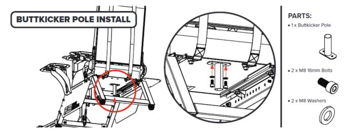
Align the mounting holes on the Buttkicker Pole with the threaded inserts under the Seat Bottom. Bolt through and secure with  $2 \times M8$  Bolts and Washers.
