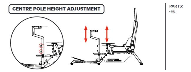
Loosen the Knobs securing the Inner Centre Pole to the Outer Centre Pole. Adjust the Inner Centre Pole to the desired height and tighten the Knobs to secure in place. Utilize the multiple threaded inserts for a perfect t.
