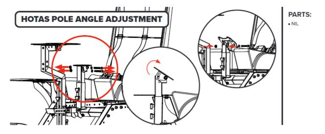
Uninstall the front Bolts, Washers and Flange Nuts securing the HOTAS Plate to the HOTAS Inner Pole. Angle to the desired position. Bolt through and secure with 1 x Bolt, Washer and Flange Nut previously uninstalled.
