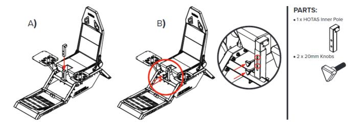
Align the threaded inserts on the HOTAS Inner Pole with the slot on the HOTAS Outer pole. Bolt through and secure with  $2 \times Knobs$ .
