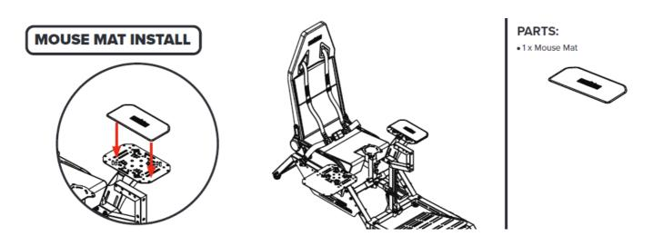
A Mouse mat may be installed ontop of the Flight or Mouse Plate. A mouse may now be used.
