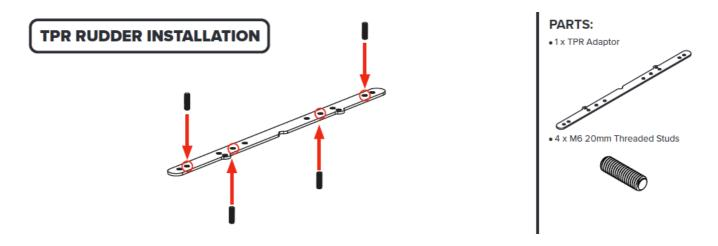
Install 4 x M6 Threaded Studs into the TPR Adaptor.
