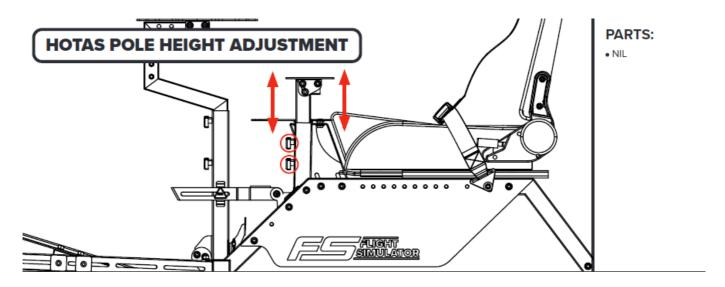
Loosen the Knobs securing the HOTAS Inner Pole to the HOTAS Outer Pole. Adjust to desired height and tighten Knobs to lock in place.
