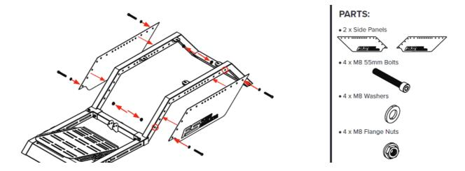
Align the mounting holes on the Side Panels with the through holes on the Seat Frames. Bolt through and secure with 4 x M8 Bolts, Washers and Flange Nuts.
