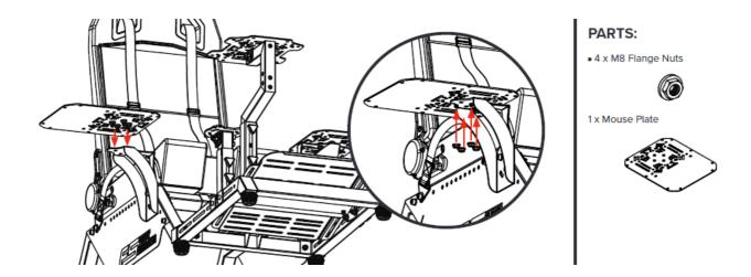
Align the Mouse Plate Threaded Studs with the mounting holes on the Straight Side Arm. Secure with  $4 \times M8$  Flange Nuts.
