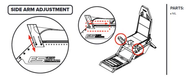
Loosen the Bolts to adjust the Side Arms to the desired height and angle. Tighten the Bolts to lock in place. Utilize the extra through holes on the Seat Frames for back and forward adjustment.
