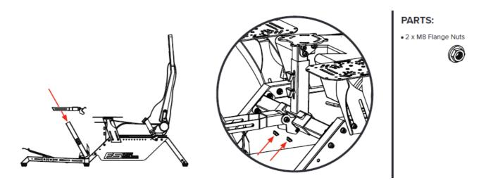
Align the mounting holes on the Support Bracket with the through holes on the Cross Member. Secure with  $2 \times M8$  Flange Nuts previously uninstalled in Step 24.
