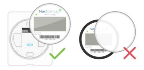
During install-on, you will disconnect the Remote Reader from the Moun-ng Plate. It is not necessary to open the Remote Reader. The Remote Reader is a sealed, watertight design, and should only be opened to replace the battery (10-year approximate bakery life).
