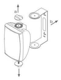
2. Using the U-bracket and a pencil, mark the hole spots for drilling in the desired position (30cm apart). Keep in mind the U-bracket only allows the W8 to rotate. Position in a way that allows you to steer the W8 later for the desired coverage.
