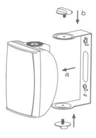
5. Select the power taps ( $8\Omega$  or 100V), connect the cables on the speaker, aim it to the desired location and tight the knob grips.
