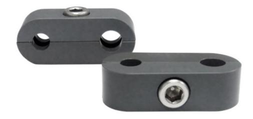
The NexSens Thermistor String Mooring Clamp Kit is designed to securely attach a string of NexSens TS210 or T-Node FR temperature sensors along a mooring line in buoy-based applications.
