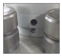
3. Install the hex screws into the holes using the included 3/16" driver to secure the S500 to the buoy plate.
