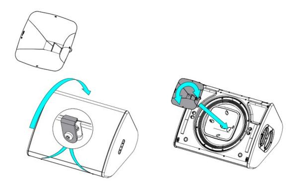
Remove the grille, and remove the flange to place the PNU-P15FLG9040. If it necessary, rotate it. Magnets keep the horn in place. Refer to the Product Data Sheet.
