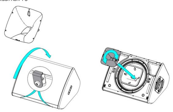
=Remove the grille, remove the flange to place the PNU-P15FLGPS. If it necessary, rotate it. Magnets keep the horn in place. Refer to the Product Data Sheet.
