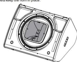
When replacing the grille, ensure it is well positioned in the top blade before fasten the hooks with the screws.
