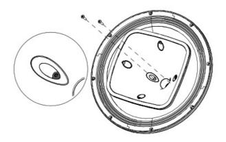
To access to the HF diaphragm, remove 4 screws. Tightening torque: 2 Nm
