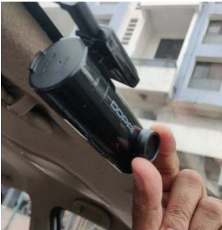
Correct Position will Eliminate Glare
